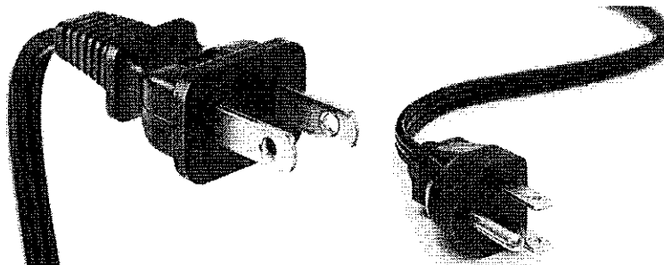
FIGURE 4. A two-prong plug is found on double-insulated tools while a three-pronged plug is found on grounded tools.
